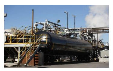
The flow of flammable/combustible material creates a friction build up during product transfer creating an electrostatic charge. Typically, transferring liquids (such as gasoline, diesel, or various grades of crude) and dry bulk products have the capability to accumulate charge.
