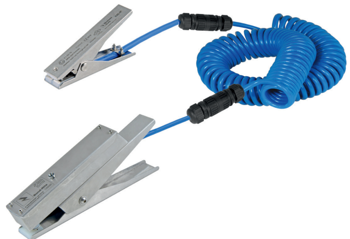
Bond-Rite® EZ with clamp mounted LED indicator that pulses green when a connection resistance of 10 Ohms or less is made between conductive portable equipment.
