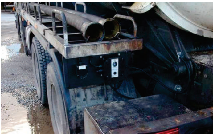
Fig 4. – The MGV system enclosure is bolted onto the side of the truck, in a locations where the LEDs are in the field view of the operators
