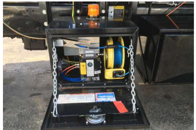
Fig 4. – The MGV system enclosure is bolted onto the side of the truck, in a locations where the LEDs are in the field view of the operators
