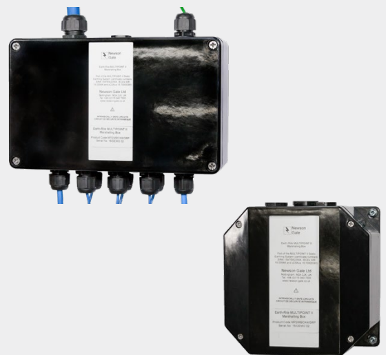
The Earth-Rite MULTIPOINT II's 4 way and 8 way marshalling junction boxes link the monitoring unit with the external ground connection points and external LED ground status remote indicator stations. The marshalling boxes can be supplied as GRP and stainless steel.
